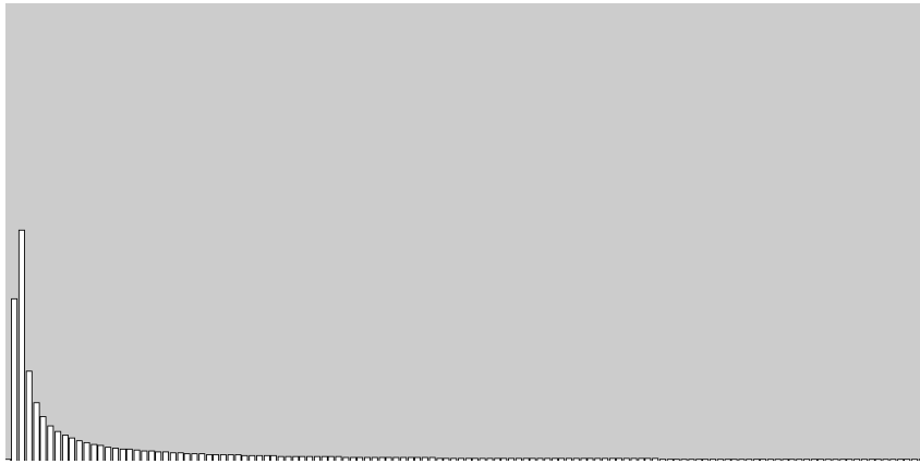
Figure 2.5.10. 8 point amplitude spectrum of f_2[t] , with spectral leakage throughout the spectrum.
