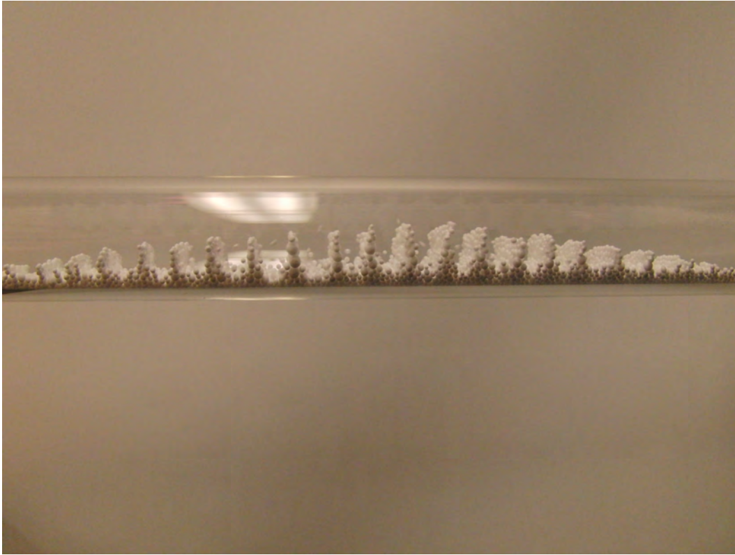
Figure 1.0.2. Kundt's tube with dust gathered at the nodes, taken from the University of Michigan Physics Department website [14].
