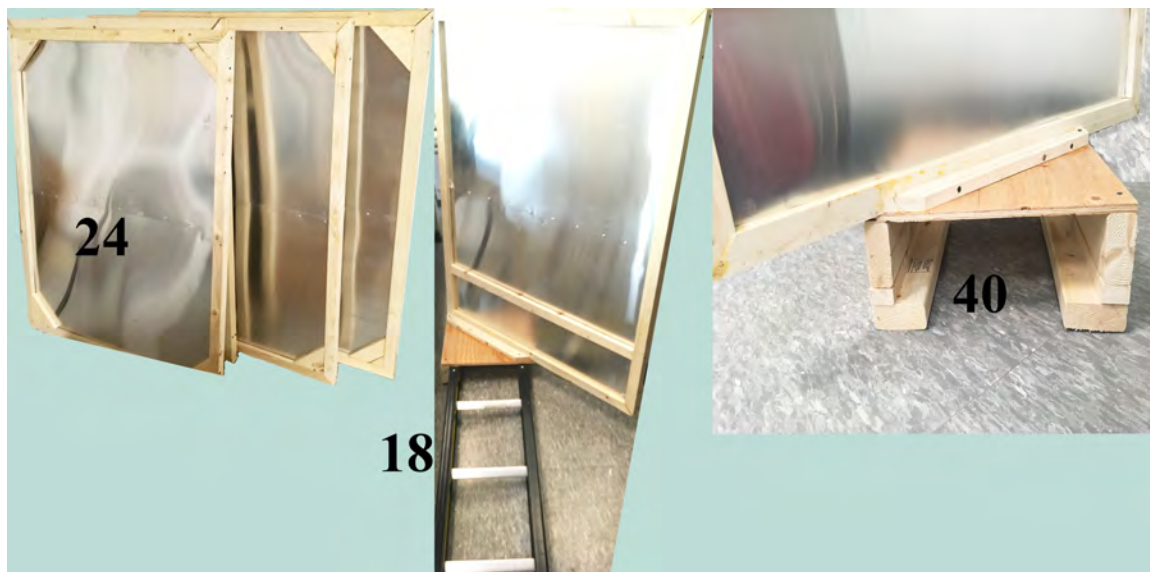
Figure 3.2.5: The mirrors are created from aluminum sheets and wooden frames similar to a stretcher bar for painting. The mirror mounts are also shown here. Notice the mount is designed to slide along the ladder.
