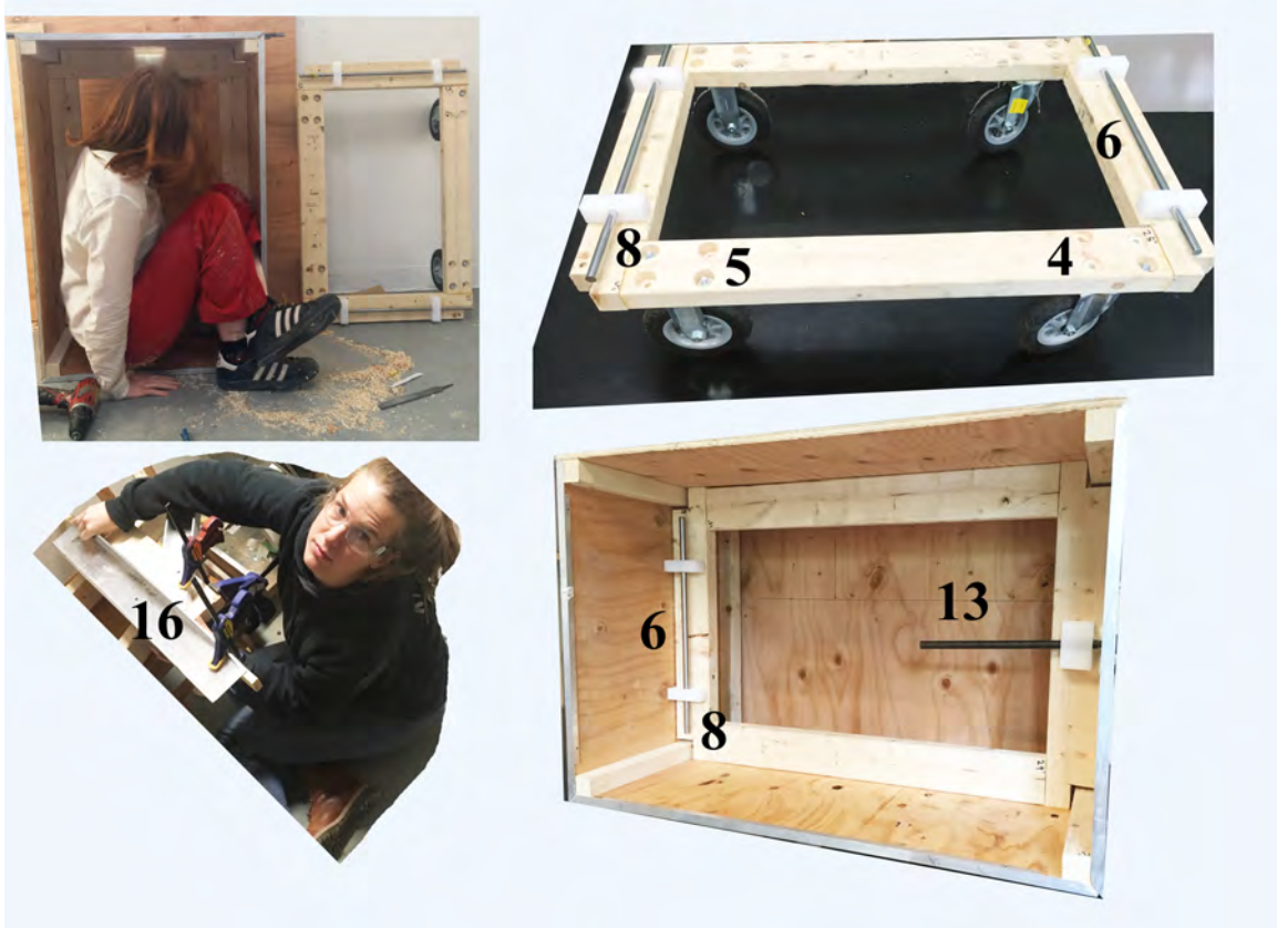
Figure 3.2.3: These photographs depict the wheels and wheel deployment system. The structure shown in the upper right photo fits inside of the box in the area shown in the lower left photo. I am chiseling a hole for the crank handle in the upper left photo. In the bottom left photo, my sister Cora is welding a support structure in a configuration to maximize strength.
