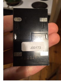
Figure 3.2.2. The back of the cell in fig 3.2.1 . The two pill shaped metal contacts half way down on the left and right are for electrically installing the cell, most commonly by soldering.
