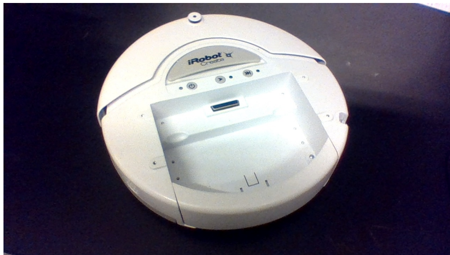
Figure 1.3.1: The iCreate v1, with its cargo port exposed
