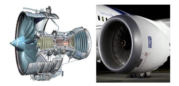
*Figure 6*. Rolls Royce turbofan engine sectioning (left) and it attached on a Boeing 787 aircraft (right).
