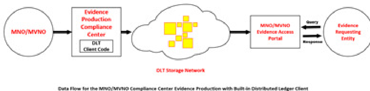
Figure 10. Data Flow for the MNO/MVNO Compliance Center Evidence Production with Built-in Distributed Ledger
