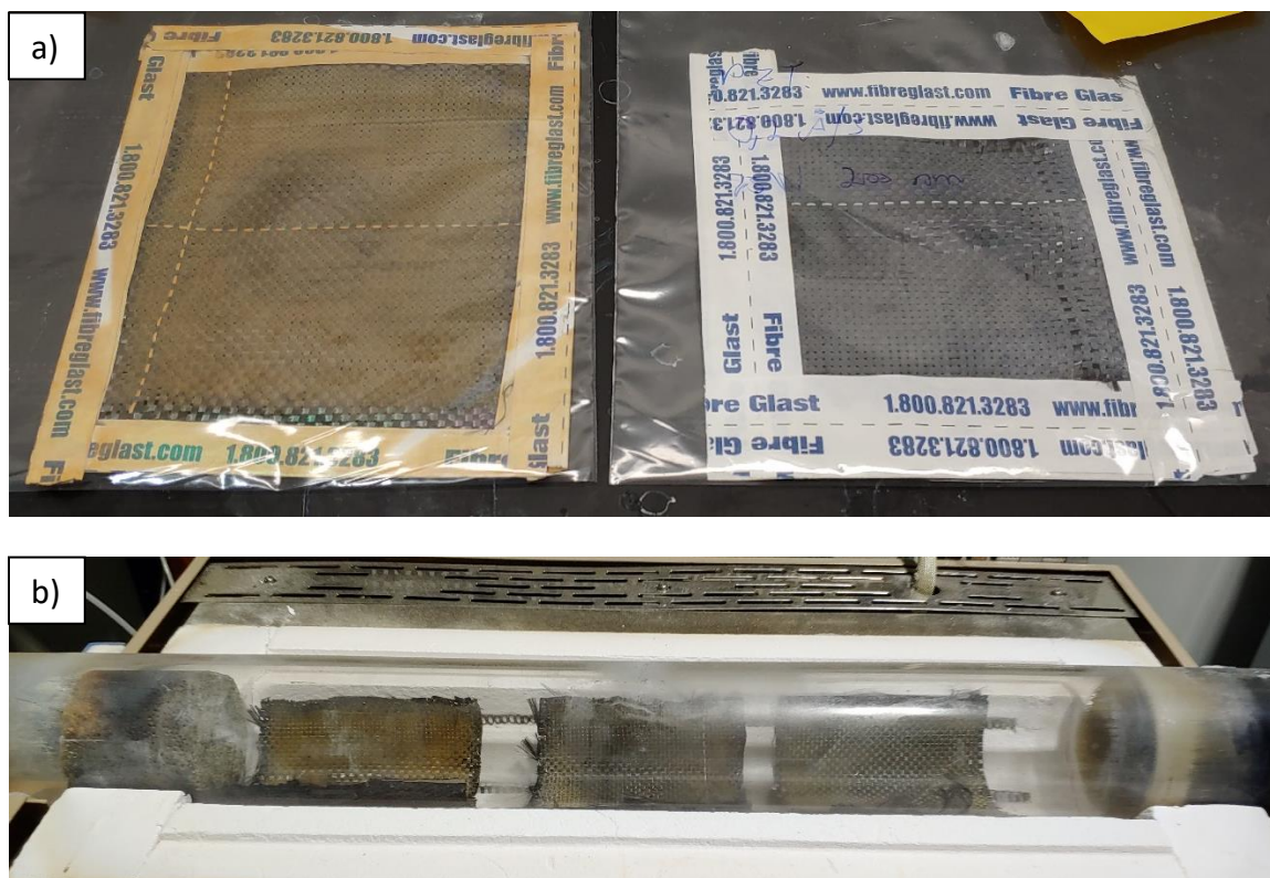
Figure 2-8. a) Left: ZnO NW sputtered with 200 nm PZT before (left) and after (right) heat treatment b) The specimens before heat treatment in the furnace tube.
