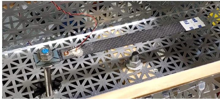
Figure 3-9. Simple CF-beam with a commercial PZT patch glued close to the clamped end
