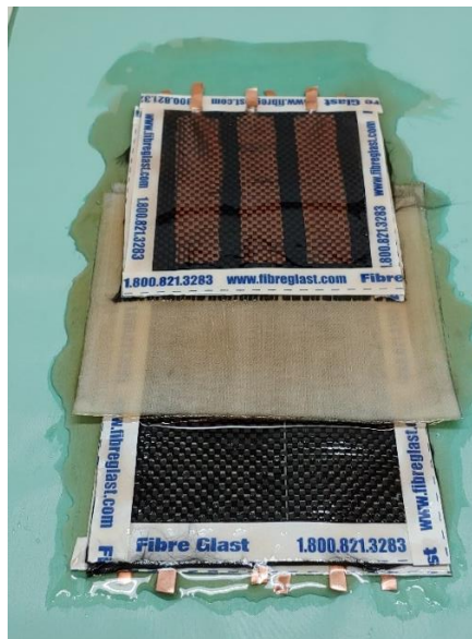
Figure 3-7. Wet layering of the stepped device with refined electrodes
