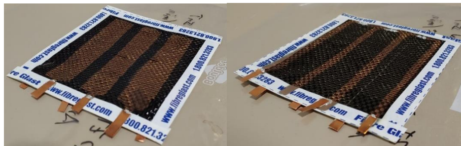
Figure 3-5. Samples after being sputtered by copper and prepared with electrodes.
