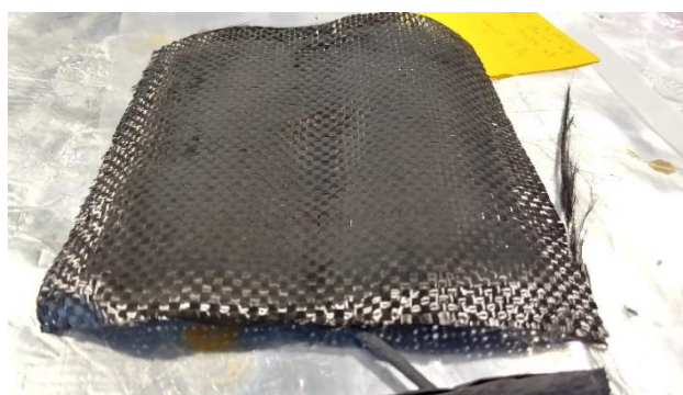
Figure 2-9. Sooted specimen after heat treatment of multiple samples together.
