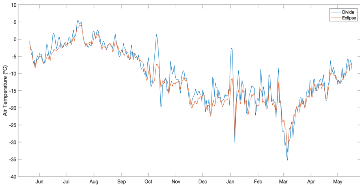
Figure 2.6 Air Temperature Records from Eclipse and Divide (May 2016 – May 2017). Divide temperatures are plotted in blue, Eclipse in orange. Plot shows daily mean air temperatures recorded by in situ instrumentation at Eclipse (iButton) and Divide (AWS).
