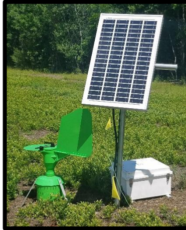
Figure 1.3. Solar powered Burkard 7-day spore trap on a blueberry barren. (Photos: Annis Lab)
