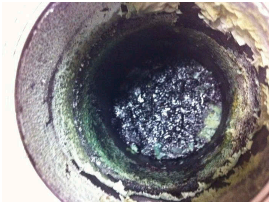
Figure 2. Corroded Parr bomb in Al-Mg-CH 3 Cl reaction.
