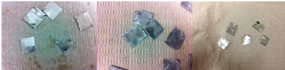
Figure 5. Fresh Al foil (left), corroded Al foil (middle) in Al- \text{AlCl}_3 - \text{CH}_3\text{Cl} reaction and foil in Al- \text{AlCl}_3 - \text{CH}_3\text{Cl} -PAG 46 reaction (right).
