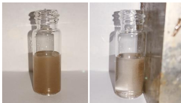
Figure 4-5 Suspended solution of CMA MNMs in water (left) and capture of CMA MNMs upon exposure to a static magnetic field (right).
