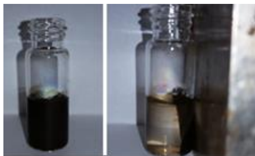
Figure 3-4 Suspended solution of CMA MNPs and capture of CMA MNPs in a static magnetic field (right).
