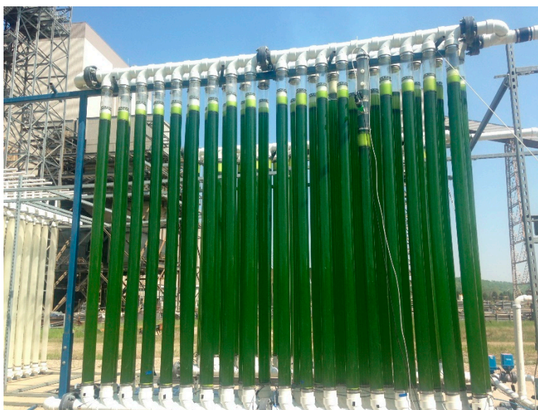
Figure 1. Cyclic flow photobioreactor (PBR) deployed at East Bend Station power plant.
