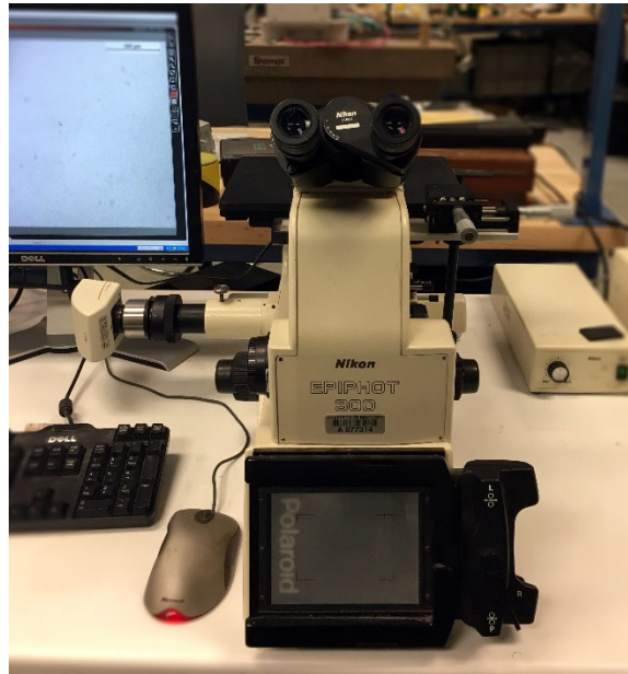
Figure 3.15 Nikon Epiphot 300 Metallurgical Microscope for surface integrity assessment
