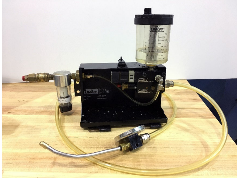
Figure 3.7 MQL delivery system
