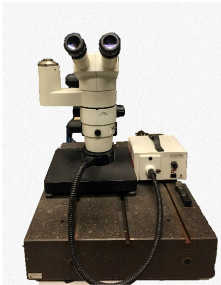
Figure 3.11 Nikon SMZ800 Microscope to measure delamination
