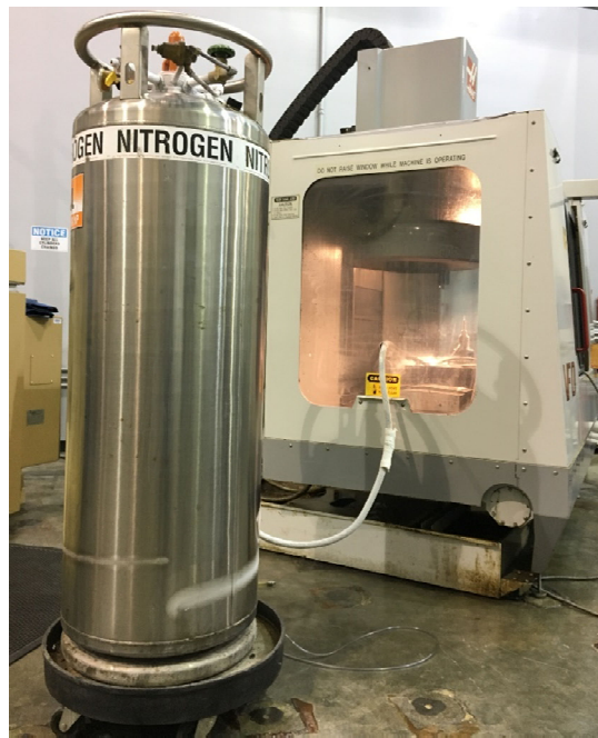
Figure 3.8 Liquid nitrogen delivery system
