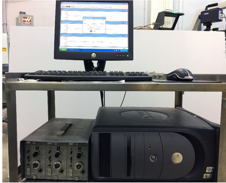
Figure 3.6 Kistler charge amplifiers connected to a computer with DynoWare software
