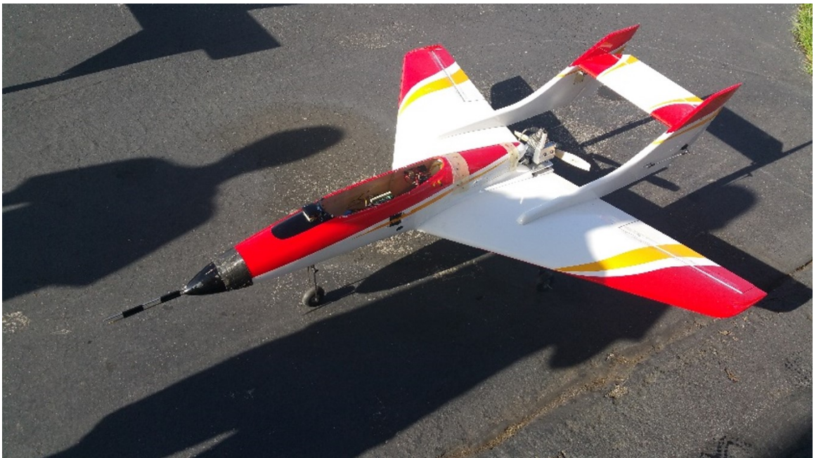
Figure 4.3: BLUECAT 3 airframe equipped with hot-wire instrumentation.
