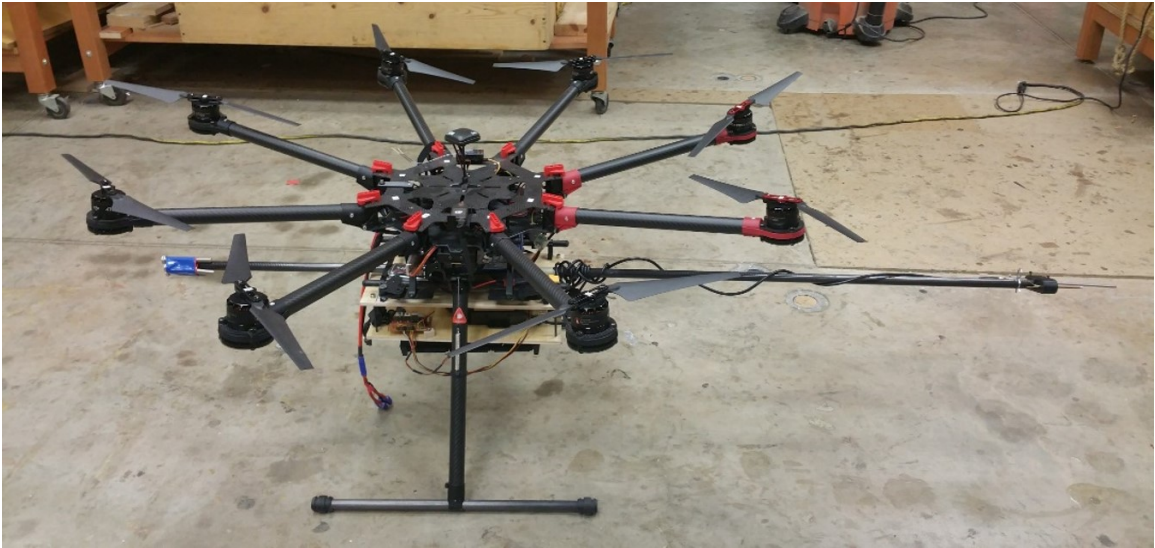
Figure 4.4: BLUECAT 4 multi-rotor equipped with hot-wire instrumentation.
