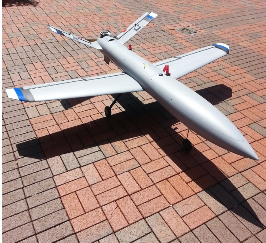
Figure 4.1: BLUECAT 1 airframe designed and built in house at the UK Unmanned Systems Lab.
