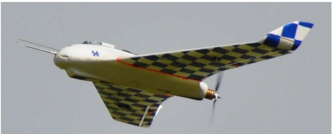
Figure 4.5: BLUECAT 5 equipped with five hole probe instrumentation.
