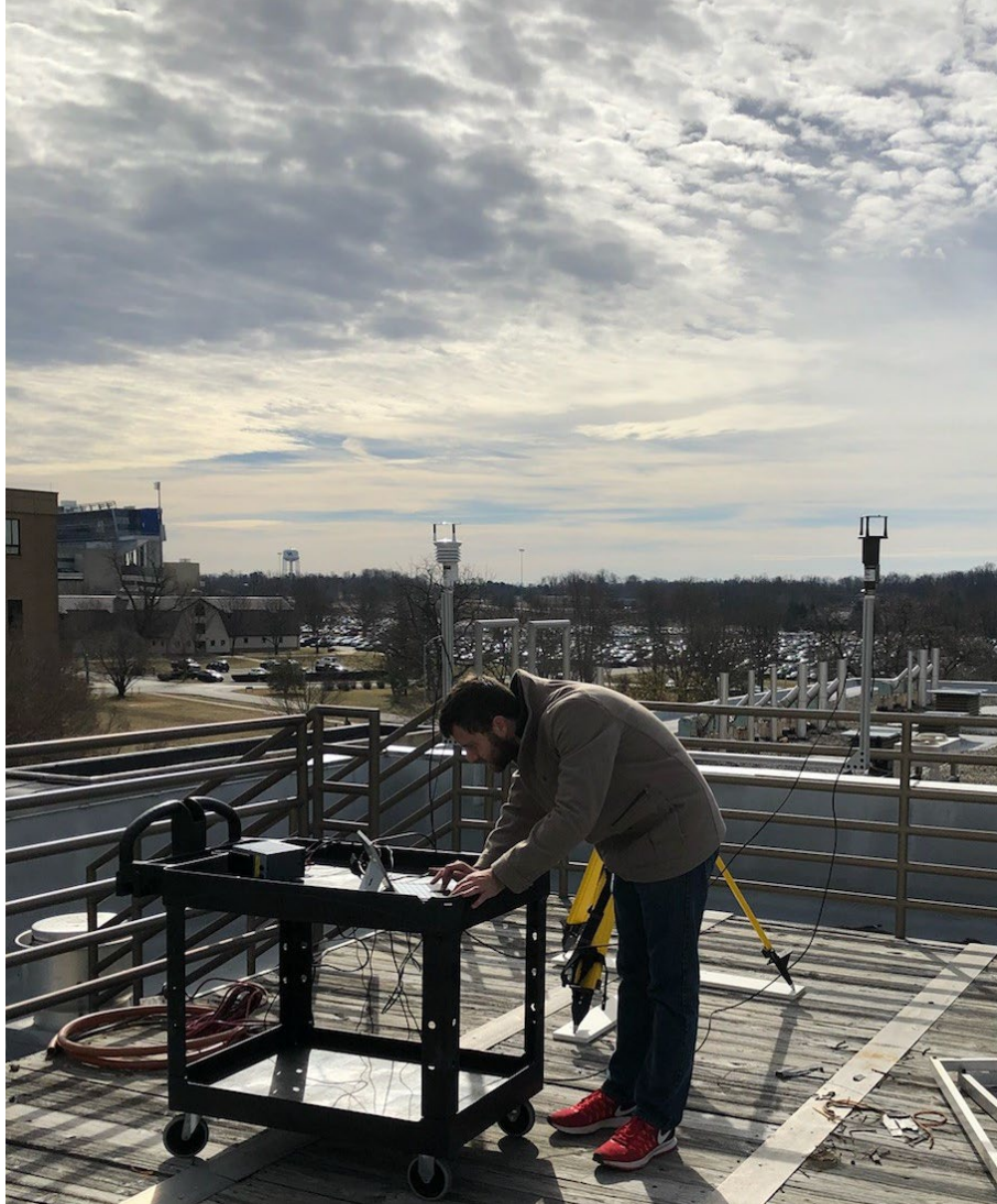
Figure 2.8 A cart was used as a surface for the computer, power supply, PCBs, and GPS receivers
