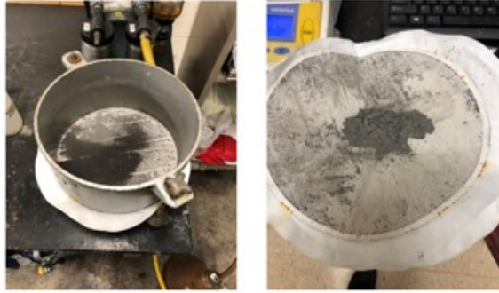
Figure 3.6: Separation of particles from the water
