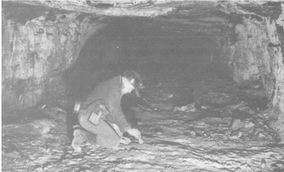
Figure 2.13: Brush and pan method sampling [83]
