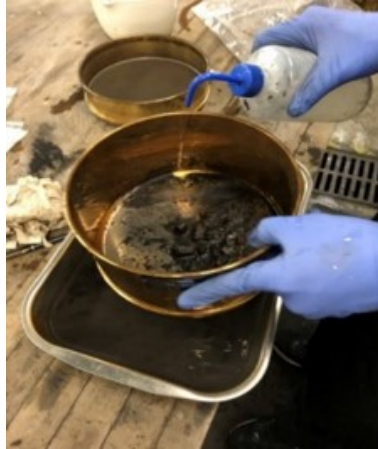
Figure 3.5: Wet sieving of particles from 200 mesh
