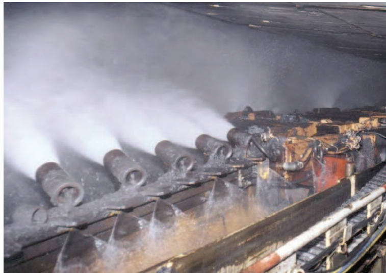
Figure 2.3: Venturi sprays directed towards coal face (Source: Dust Control Practices for Underground Coal Mining, CDC, NIOSH.)
