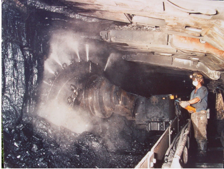
Figure 2.6: Water sprays on longwall shearer (Source: CDC, History of the Mining Program)
