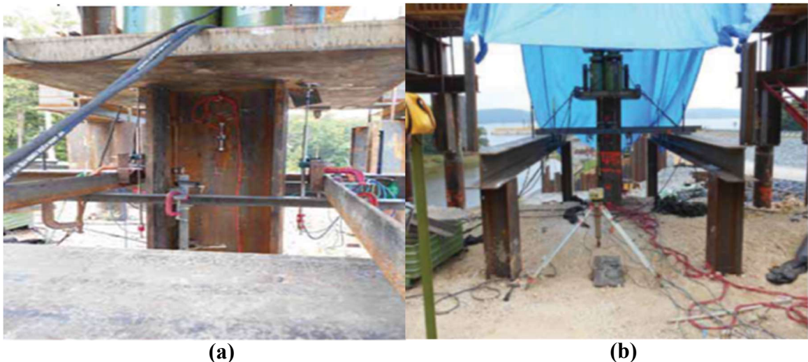
Figure 17. Head Movement Measurement: (a) Pressure Transducers; (b) Reference Beam
