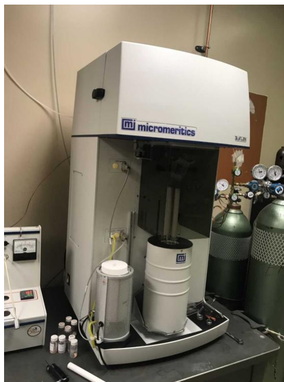
Figure 15. Instrumentation used for surface area and pore volume analyses.
