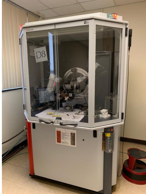
Figure 14. XRD instrument used for mineralogy analysis.
