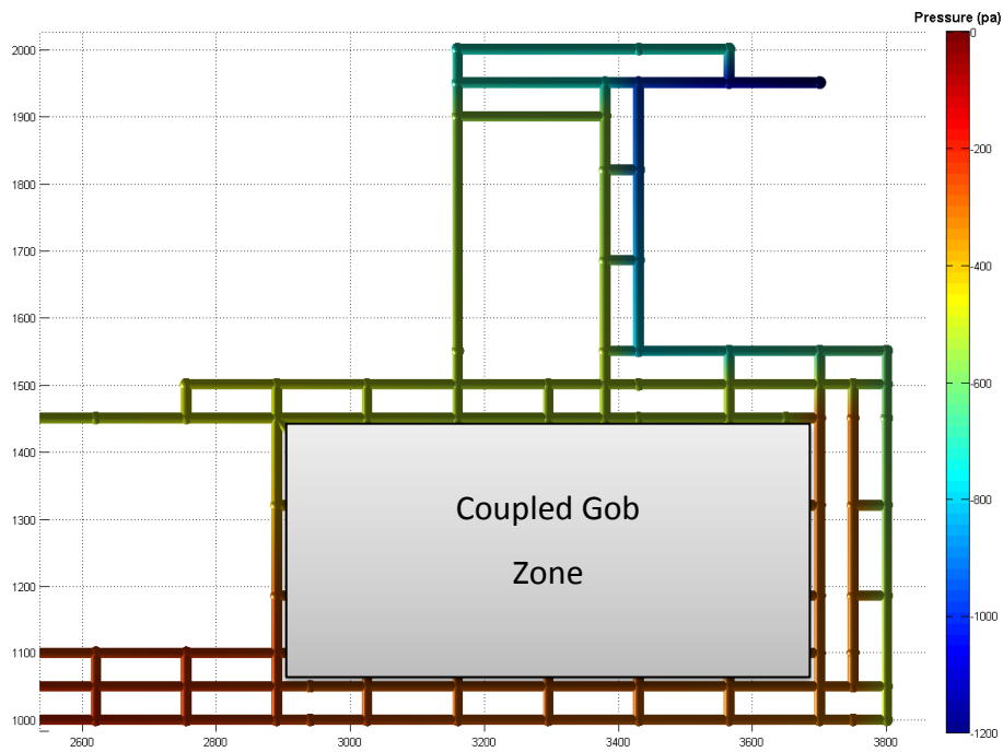
Figure 4-16 Pressure through the network when coupled with the level 5 mesh
