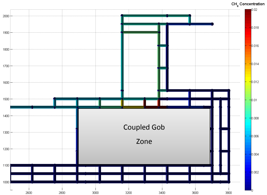
Figure 4-38 Network model response to methane addition at the longwall face
