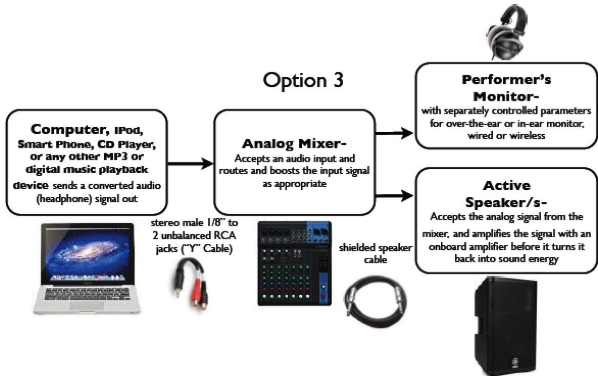
Figure 8. Basic Electroacoustic Audio Paths Relevant for Tape Works-Option 3, Mixing Board with Performer Monitor.
