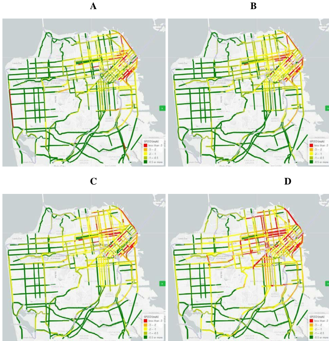
Figure 13 Speed (mph) difference between 2016 scenario with TNCs and a counterfactual 2016 scenario without TNCs for (A) 6-9 AM, (B) 9 AM-3:30 PM, (C) 3:30-6:30 PM, and (D) 6:30 PM-3:00 AM.
