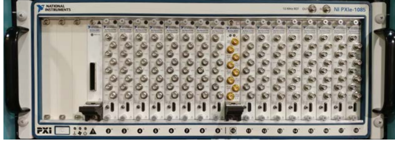
Figure 5.2: A photograph of the instrumented primary DAQ chassis. The secondary chassis contains identical hardware, with the exception of the timing module installed in slot 10.
