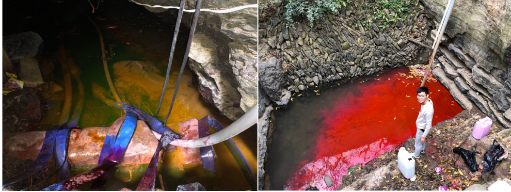
Figure 14: Field photographs showing winter baseflow dye injections at Sanjianfang (left) and Daxing (right).
