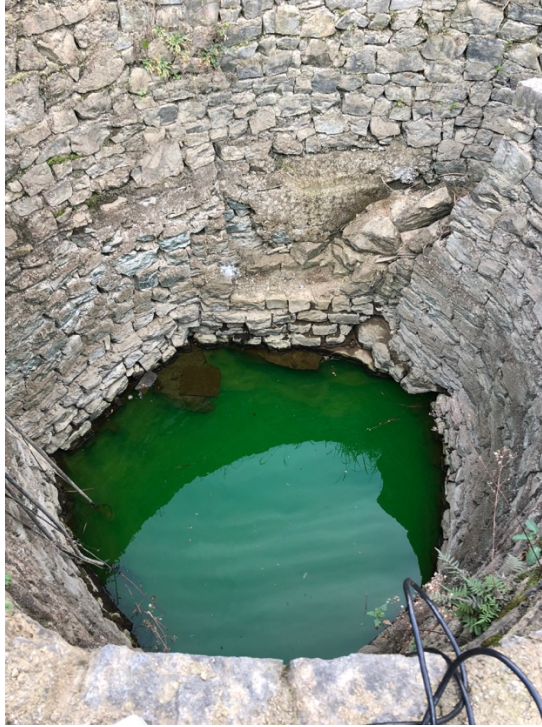
Figure 55: Field photograph of Xiao Shanba on December 3. Note the green color suggestive of residual fluorescein.
