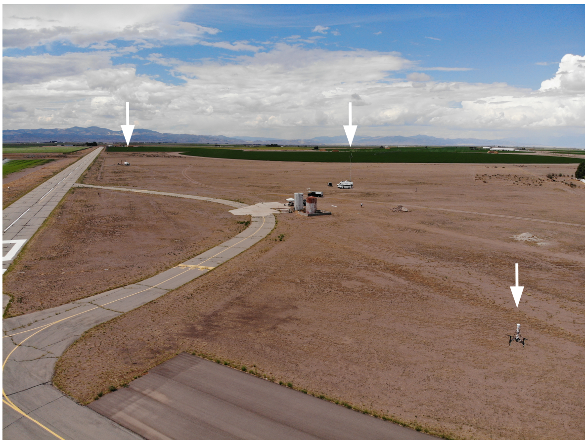
Figure 4. Simultaneous flights with sensors in a triangle formation (white arrows). Both UASs were operating off of marks on the taxiway, and the MURC tower was stationed north of the UAS operations.
