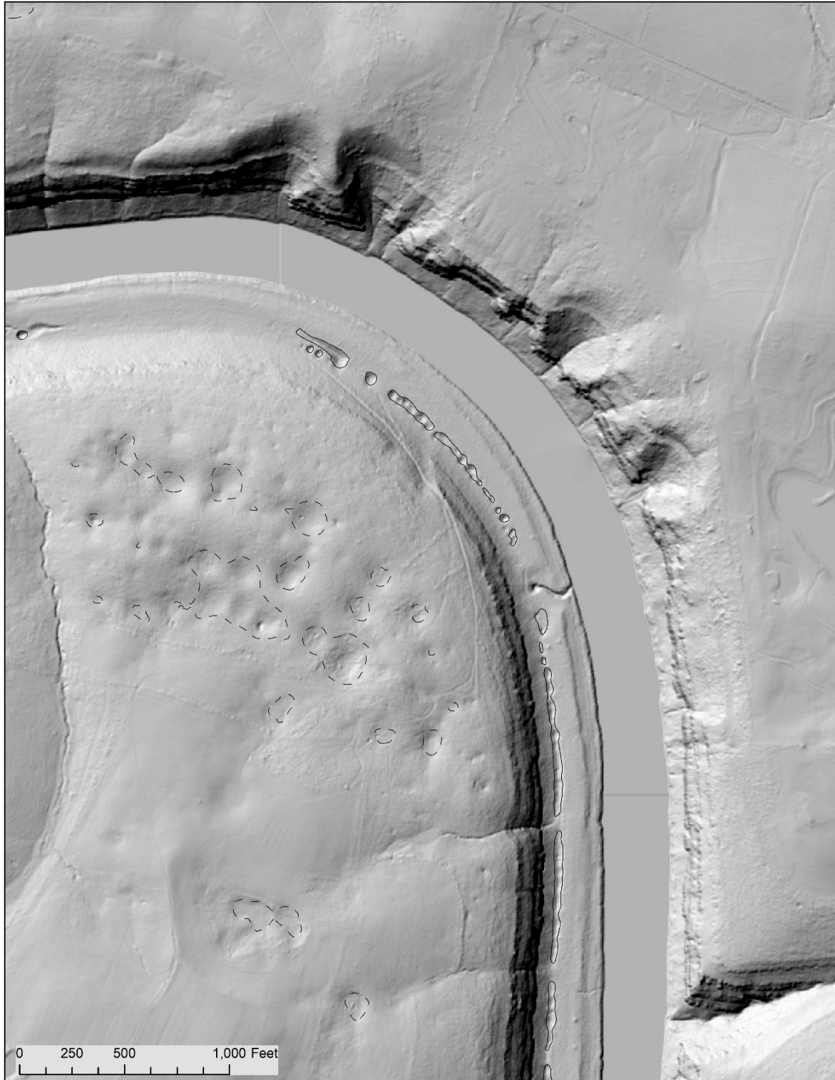
Figure 2. A hillshade of a section of the Kentucky River derived from LiDAR data. The depressions near the river (outlined solid black) are a typical example of the unusual depressions found in the alluvium of some of the major rivers in Kentucky. The depressions on top of the hill (outlined in dashed black lines) are sinkholes.
