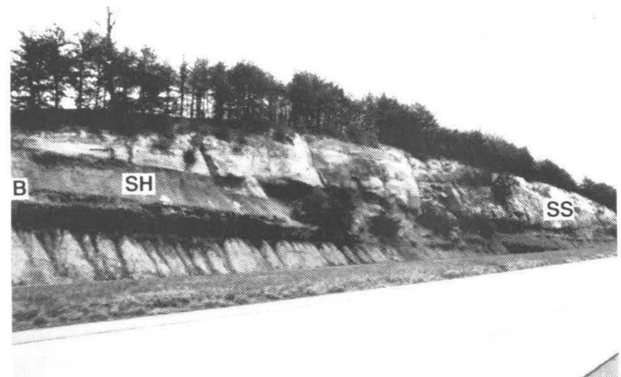
Figure 40. Springfield coal exposed on the Western Kentucky Parkway near milepost 32. The coal is 1.5 m (4.9 feet) thick and is overlain by a high-resistivity, bony shale (B) with pelecypod and brachiopod fossils; a dark-gray, silty shale (SH); and a thick sandstone (SS).
