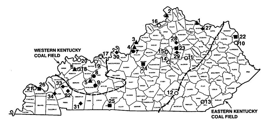
Figure 1. Map of Kentucky showing: (1)  $SO_2$  emission control strategy of coal-fired electric utility plants [flue-gas desulfurization (FGD) or burning low- and medium-sulfur coal], (2) atmospheric fluidized-bed combustion plants, (3) sources of stone for  $SO_2$  emission control, and (4) coal fields. Modified from Enoch (1983). Explanation for Figure 1 on following page.
