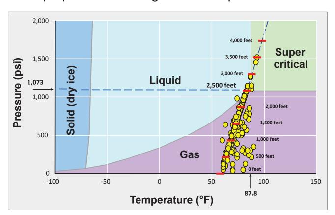
This graph shows the phases of carbon dioxide (CO<sub>2</sub>) at different pressures and temperatures. The yellow dots represent pressures and temperatures recorded from wells drilled in Kentucky. Pressure and temperature increases with depth. At surface pressure and temperature, CO<sub>2</sub> is a gas. At a pressure of 1,973 psi and temperature of 87.8°F, CO<sub>2</sub> is a supercritical fluid. This pressure and temperature occur at depths of approximately 2,500 feet in Kentucky.
