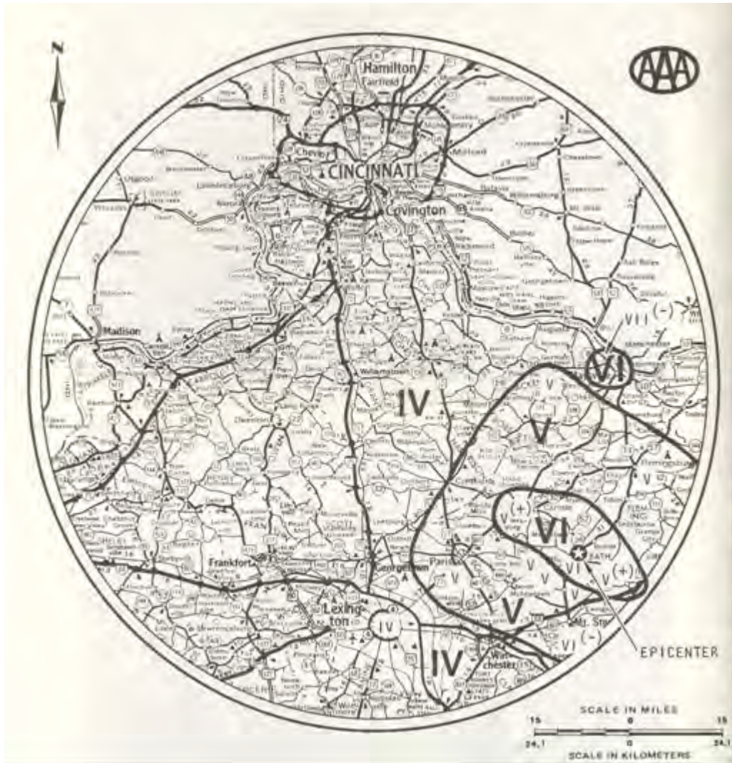
Figure 1-6. High MMI in Maysville was caused by amplified ground motion during the 1980 Shapsburg earthquake. From Hanson and others (1980).
