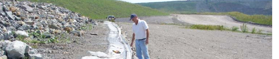
The University of Kentucky College of Agriculture has studied the growth of trees on coal mine spoil piles for several years. These spoil piles have been shown to sustain phenomenal tree growth over a very short time span. Here, aprons have been applied at the base of spoil piles made of different rock types to monitor sediment loss as rainwater filters through the pile. Photo by Bart Davidson, Kentucky Geological Survey.
