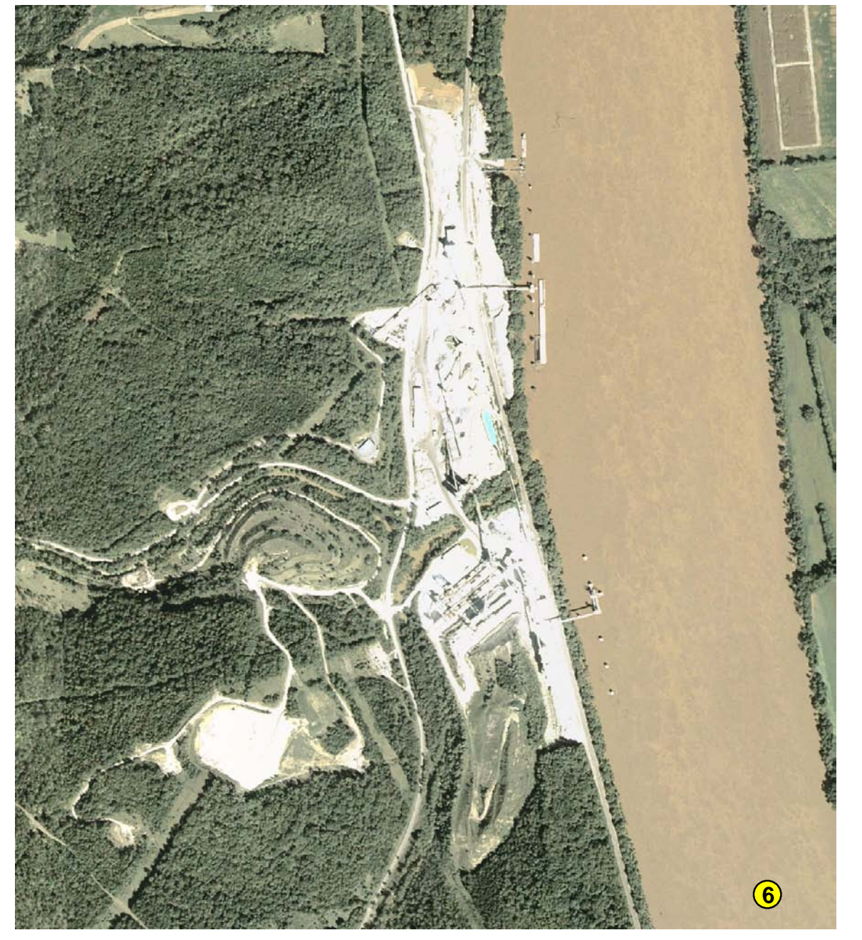
Carumee Lime produces 1.4 million tons per year of high-calcium lime for power plant scrubbers and the steel industry from its 600-foot-deep slope mine on the Ohio River. Aerial photo (2004) by the U.S. Department of Agriculture, Farm Services Administration, National Agricultural Imagery Program.
