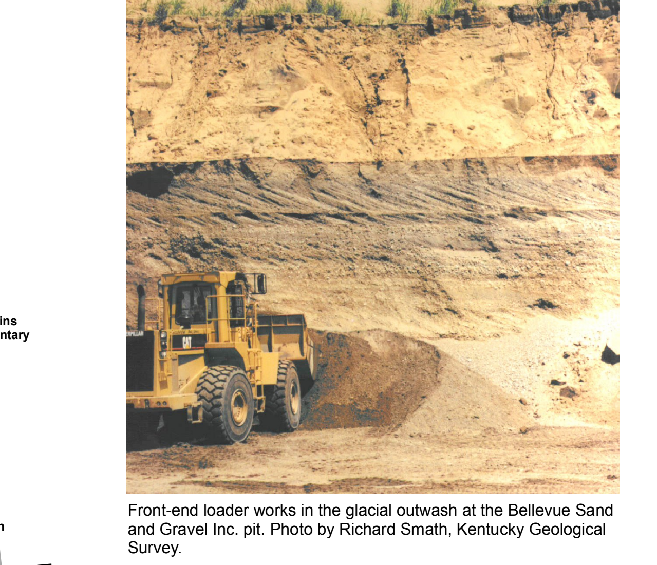
Front-end loader works in the glacial outwash at the Bellevue Sand and Gravel Inc. pit. Photo by Richard Smath, Kentucky Geological Survey.
