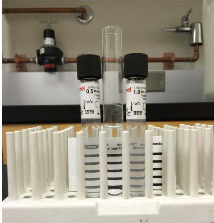
Figure 3.8: Test Tube with Water, McFarland Standards and Wickerham Card; ThermoFisher Scientific, Waltham, MA.
