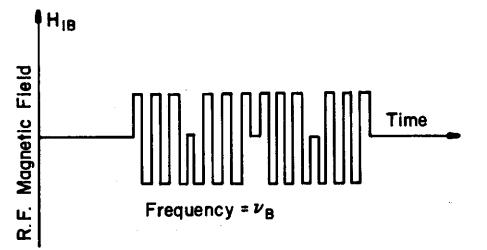
The B nuclei are irradiated with an rf field intensity  $H_{1B}$  at the time points (b) to (c), lasting for a time  $\tau_0$  of the order of  $T_{1d}$ , indicated in Fig. 1. The double resonance cross-relaxation rate  $R_{AB}$  which is a measure of the transfer rate of spin ordering from the A to the B system is greatest when
