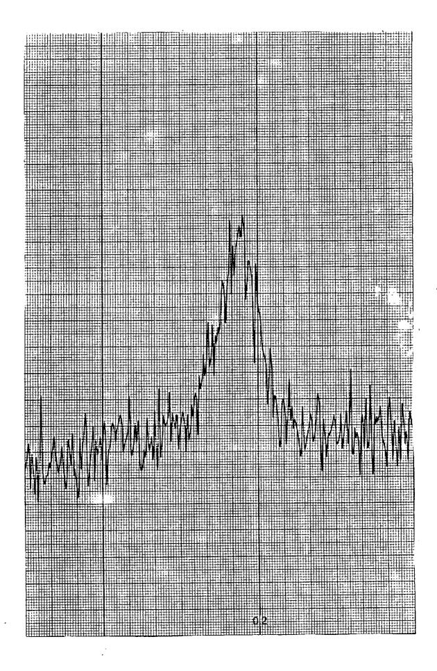
Fourier Transform representation of the chlorine signal of carbanolate after signal averaging (concentration 20 ppb).
