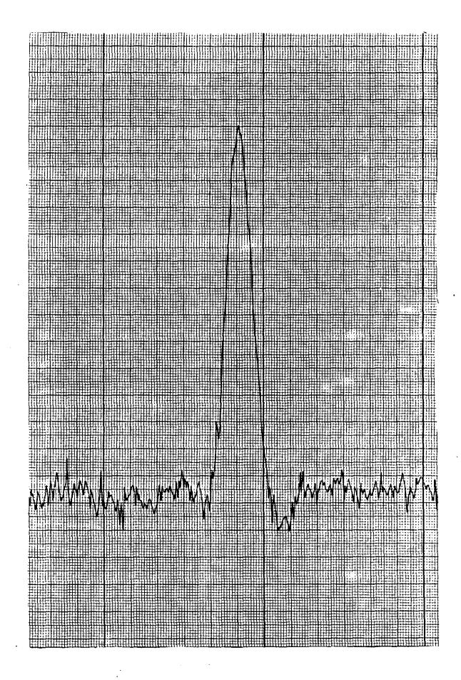
Fourier Transform representation of the chlorine signal of carbanolate after signal averaging (concentration 100 ppb).
