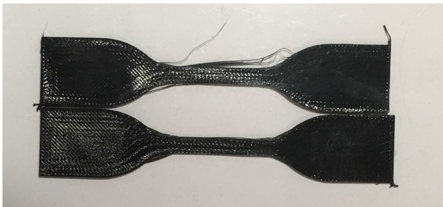
Figure 3.36: Specimen folding at Instron initial position, indicating permanent deformation
