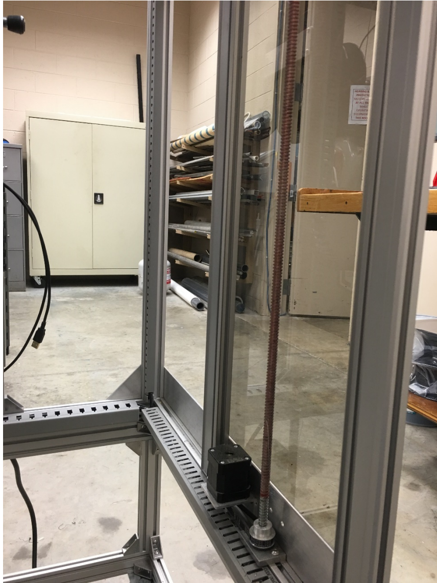
Figure 1.7: FFD printer “Z” travel mechanism
