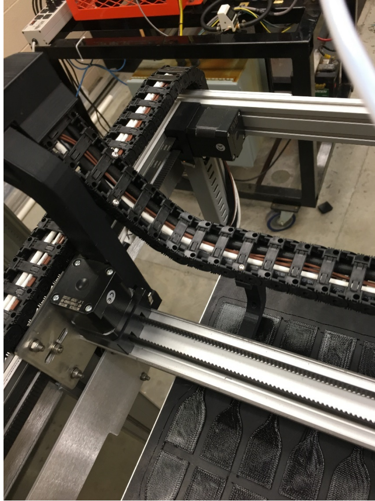
Figure 1.6: FFD printer “X” and “Y” travel mechanism
