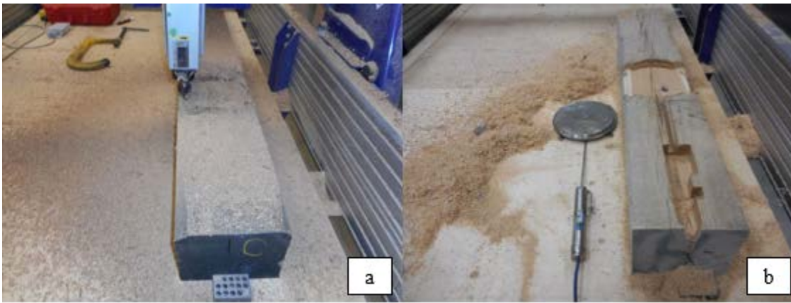
Figure 3.7 Routing the Pressure Cell Recess
