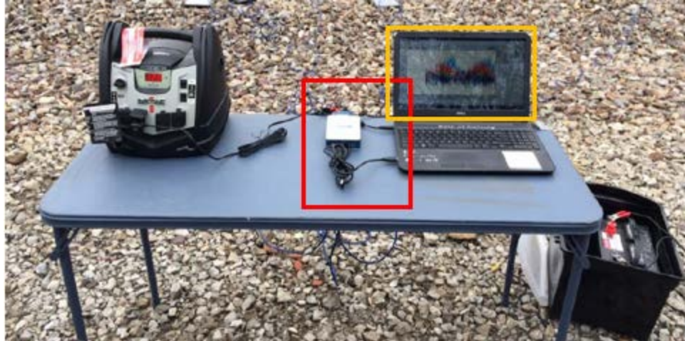
Figure 3.5 Pressure Test Setup
