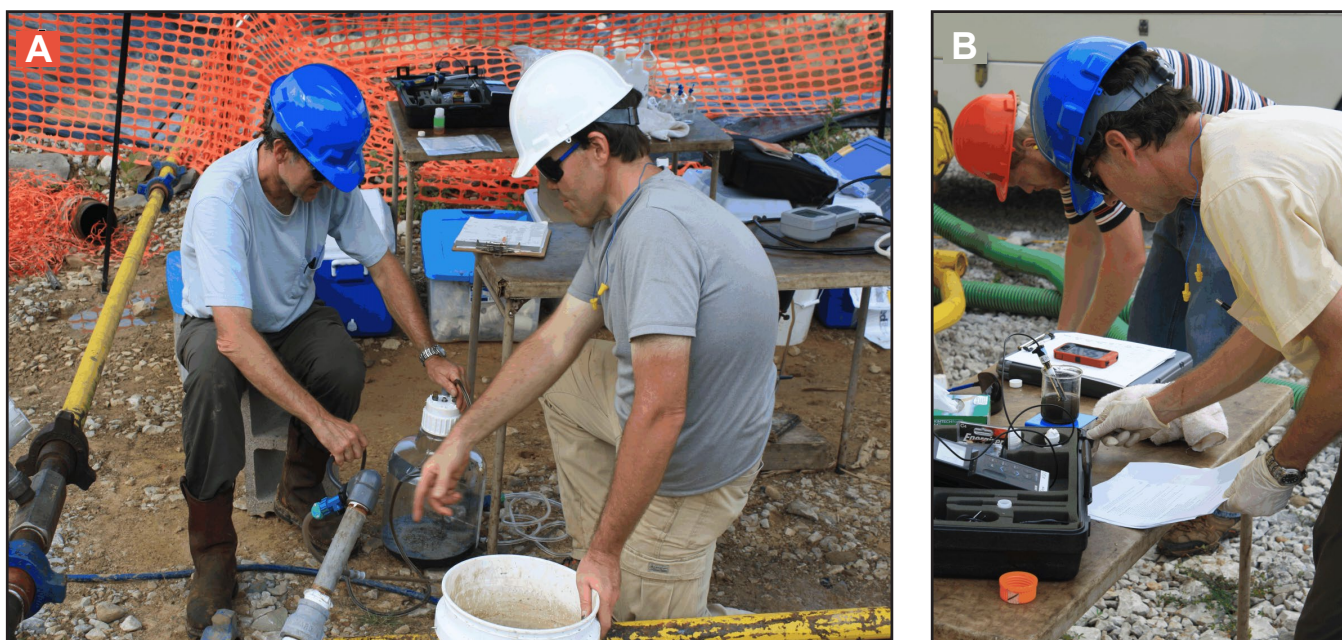
Figure 18. KGS geologists sample formation water swabbed from a step-rate test interval prior to testing. (A) Marty Parris (left) and Steve Webb connect a carboy to collect a water sample. (B) University of Kentucky Department of Earth and Environmental Sciences student Jerry Grider (left) and Marty Parris monitor water-sample conductivity before collecting a sample.
