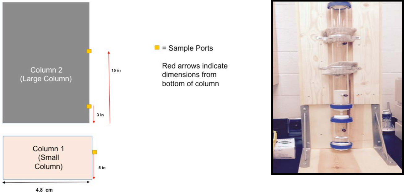
Figure 1. Soil Column Schematic (Left) and Photo (Right)
