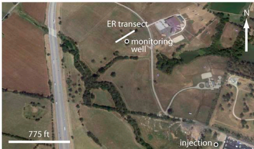
Figure 1: Map of injection site, monitoring well, and electrical resistivity transect at the Kentucky Horse Park in Lexington, KY.
