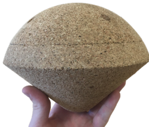
Figure 3.4: Final assembly of the KRUPS capsule for the KUDOS mission
