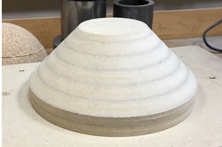
Figure 4.4: KOREVET support (made out of MDF) used to stabilize cork as it was machined
