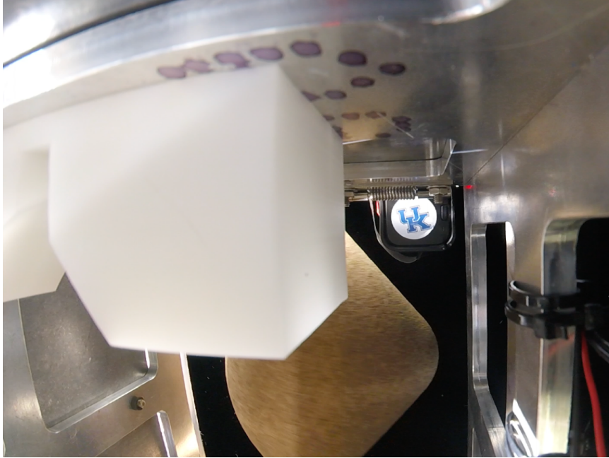
Figure 3.18: Video screenshot as the capsule is being ejected from KREM at rocket apogee (150 km)
