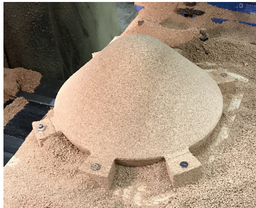
Figure 4.5: KOREVET TPS bottom shell during the machining process
