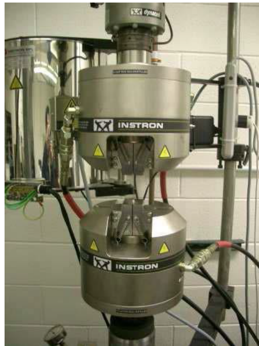
Figure 2.3. The Instron 8800 servo-hydraulic machine for tensile test.
