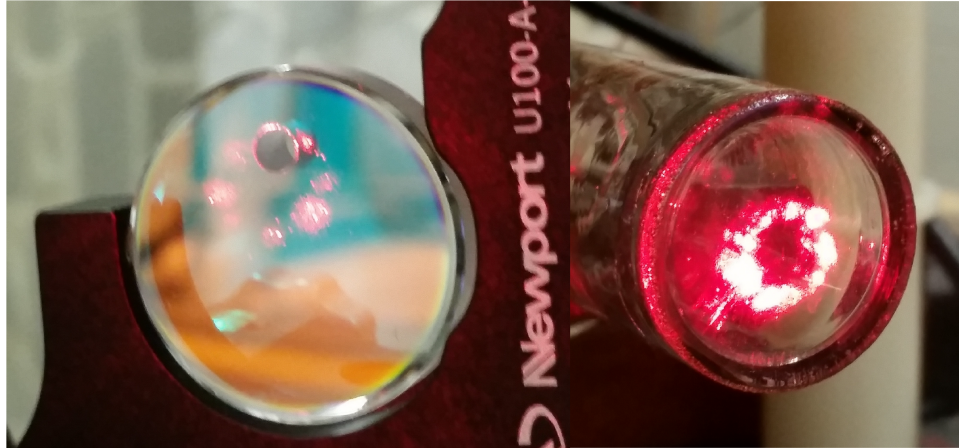
Figure 5.12: 13 pass beam spot pattern on the surface of the end window for Vivian and on the surface on the mirror.
