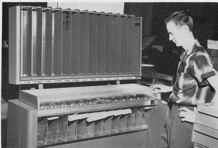
Figure 6.—IBM Type-083 (Sorter). The bid data cards from the 533 are next merged with their respective bid item description cards, which were prepared in Figure 1 and Figure 2. This merging process is accomplished by the sorter, which sorts at the rate of 1,000 cards a minute.
