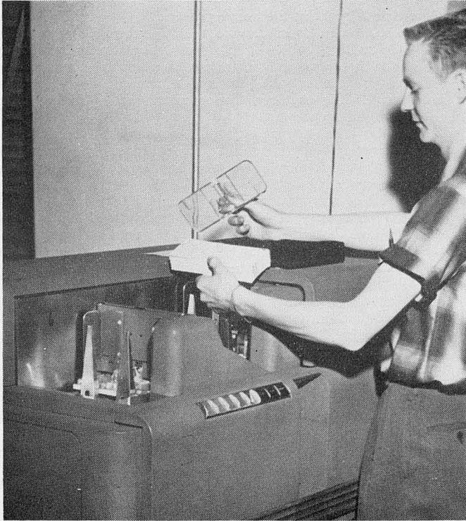
Figure 2.—IBM Type-514 (Reproducer). Using the deck of cards assembled in Figure 1, the operator next uses the reproducer. Here bid item descriptions are automatically reproduced from the master cards into the respective bid item cards. This operation is also completed one or two days before the bids are opened. The bid item cards are filed in a drawer to be used on the date the bids are opened.
