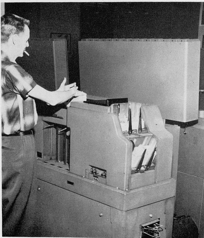
Figure 1.—IBM Type-077 (Collator). The operator is merging bid item cards with their respective master cards. This operation is performed one or two days before the bids are opened.
