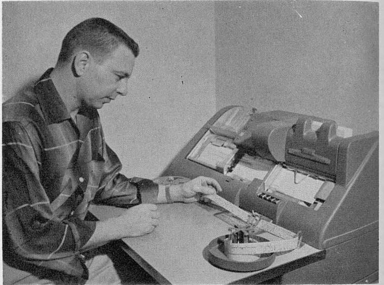
11. Tape to card punch. Data are recorded on perforated paper tape in the field and transferred to punched cards in the processing center.
