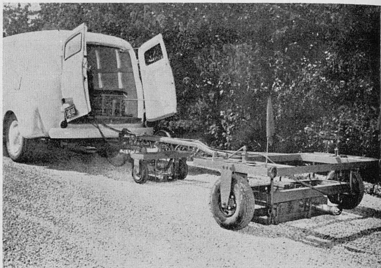
Fig. 4—Continuously recording nuclear moisture-density logging unit for highway work.
