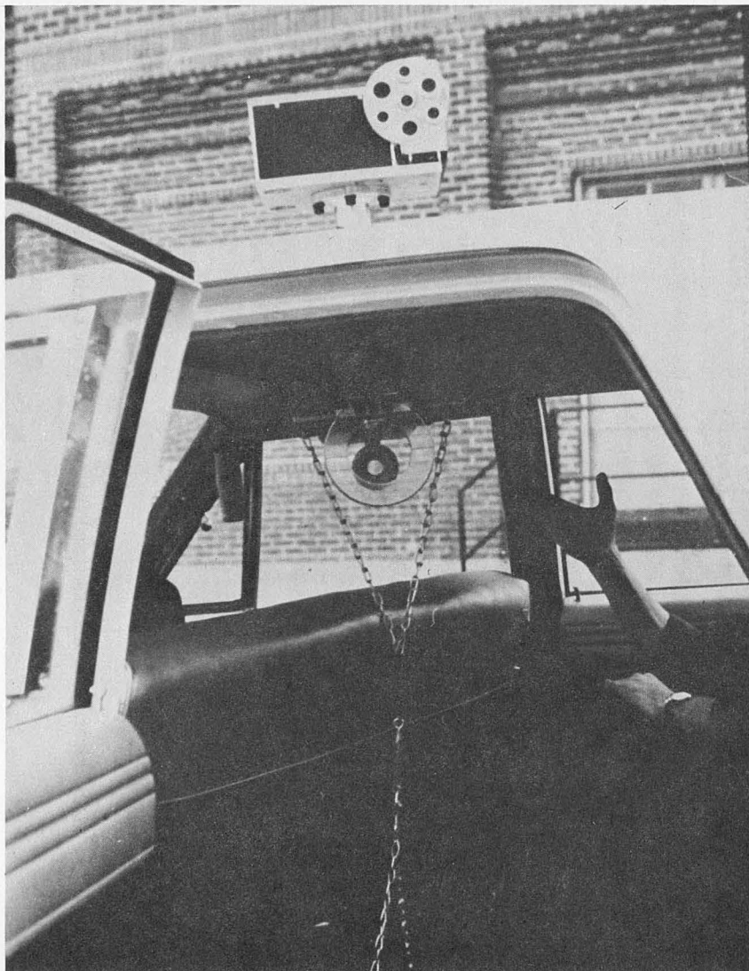
Figure 40. Automobile-Mounted Aiming Device and Remotely Controlled 16 mm Camera Used in Filming Driver Errors for Use in the Televised "Traffic Madness" Driver Re-education Program
