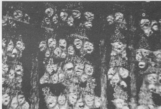
Figure 12. Cross Sectional View of Dark Wood from Pier No. 2, Magnified 17.5X. Note greater abundance of large pores; specimen contains 17.5 rings per inch and 10 rays per inch.
