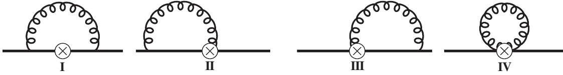
FIG. 1. Feynman diagrams for the calculation of Z_{Q \to Q} . The circle represents an insertion of the twist-2 operator.
