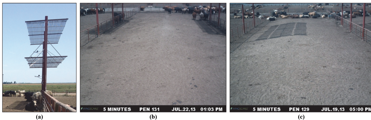
Figure 8. (a) Positions of the black globes and (b) shade acting as a double layer creating less shaded area but potentially greater solar reduction and (c) shade acting as a single layer with greater coverage area but potentially less solar reduction.
