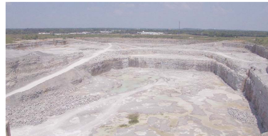
Limestone is an abundant rock in Christian County. One of several active quarries in the county, the Roggins Group Hopkville Aggregate Quarry, shown above, produces approximately 1.5 million tons of crushed stone per year. Photo by Glynn Beck, Kentucky Geological Survey.
